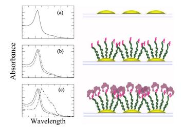
FIG. 7. (Color online) Schematic of proposed NP chain on waveguide sensor. (a) HGNP's immobilized on a transparent substrate give rise to a single particle spectrum. (b) GNPs after functionalization with recognition sites lead to a slight redshift in the spectral peak. (c) Binding the analyte to the recognition sites leads to a huge spectral change—NP-like to nanowirelike—due to the onset of cross-talk.
