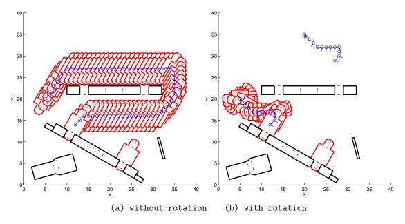
Figure 6: Collision-Free Moving Paths without/with Rotation
