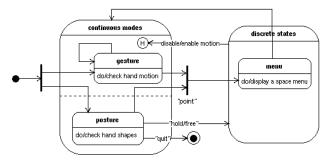
Figure 1: State Transition Diagram of "Hand"
