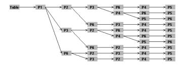
Figure 5: The Assembly Tree of the Die-Set
