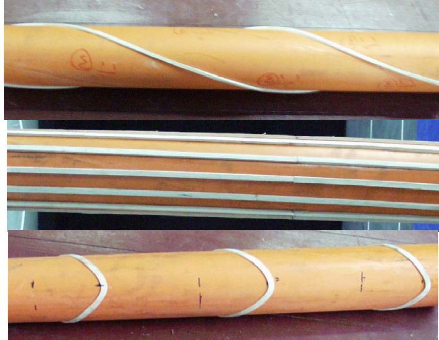
Figure 2-7 Illustration of different types surface protrusions
