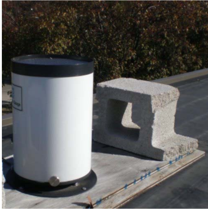
Figure 3- 6: Isco Tipping Bucket Raingauge
