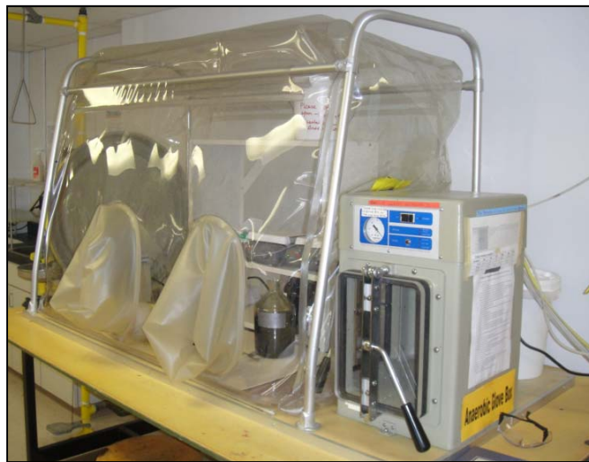
Figure 3.1: Coy® anaerobic chamber
