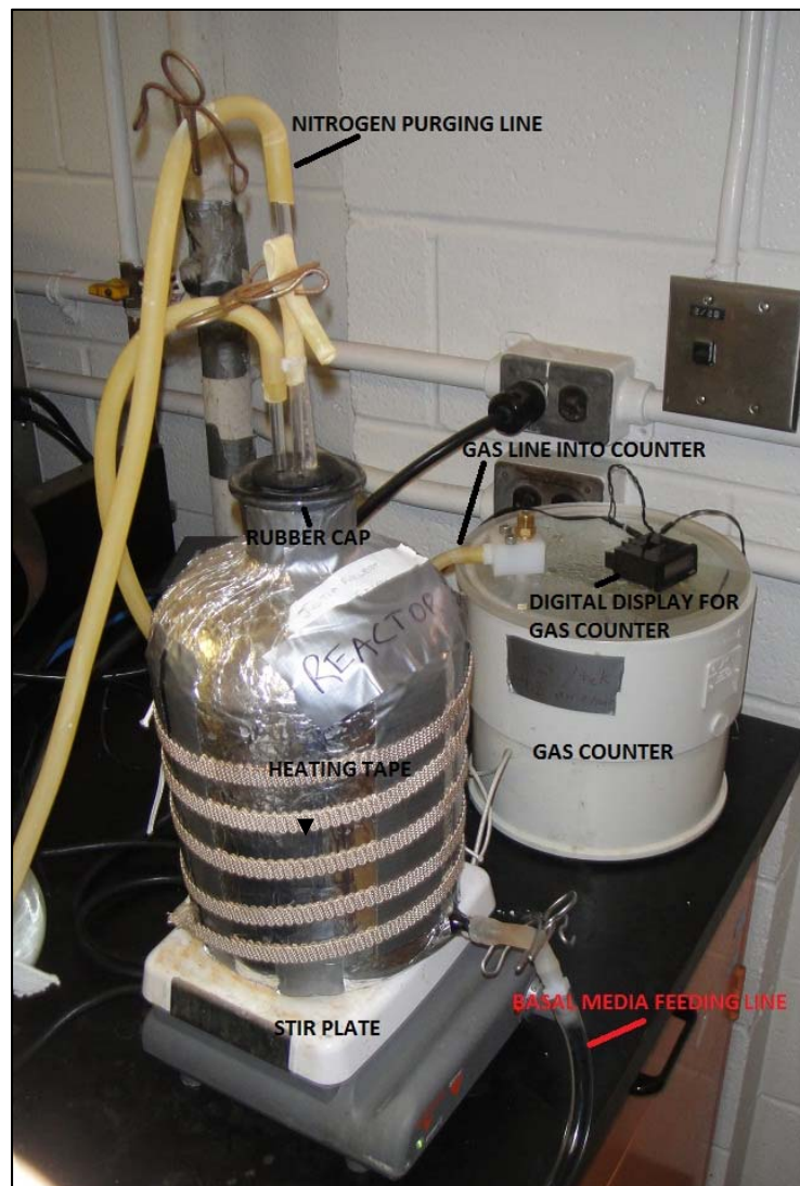
Figure 3.3: Reactor Set-up
