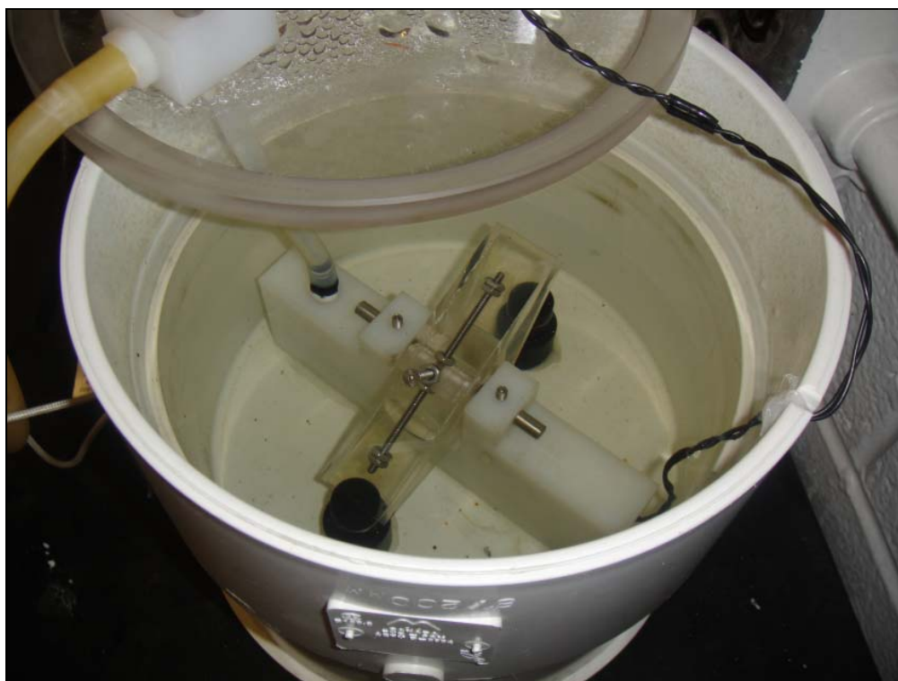
Figure 3.4: Internal View of Gas Counter
