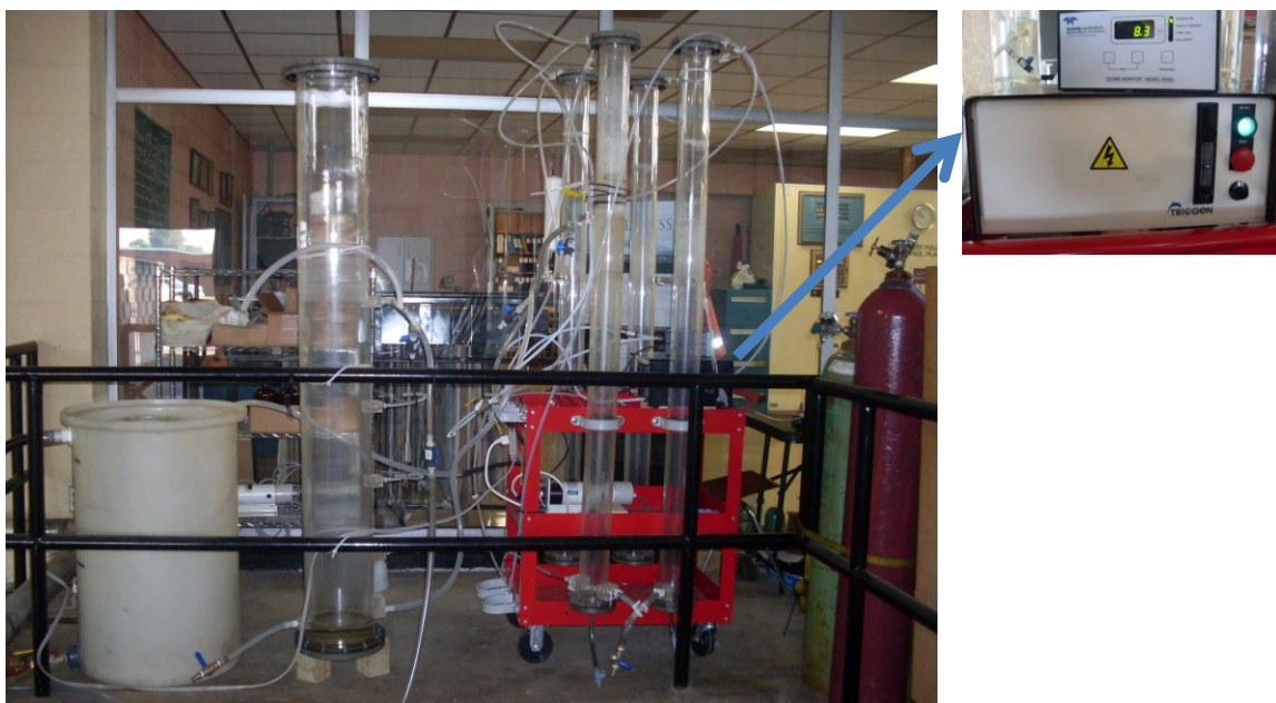
Figure 3.3 Picture of the pilot unit installed at LRPCP (inset picture shows the ozone generator and monitor)
