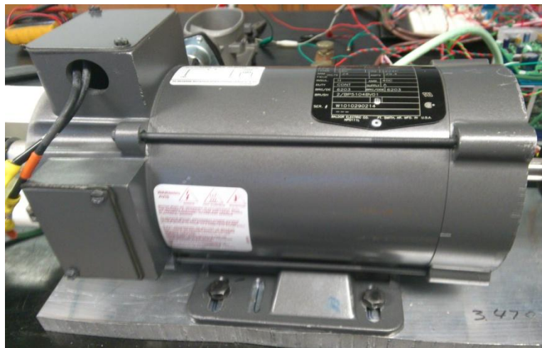
Figure 4-3 The Baldor Motor used to test the disturbance torque estimator
