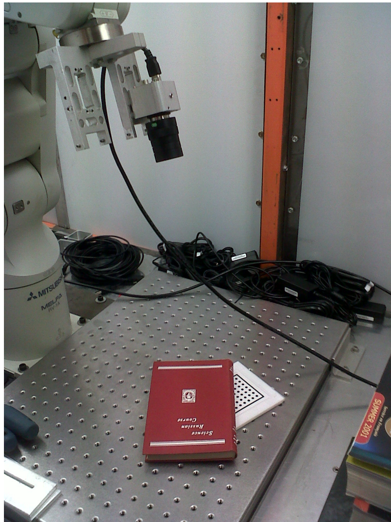
Figure 4.16: Target occluded by the obstacle in the vision platform
