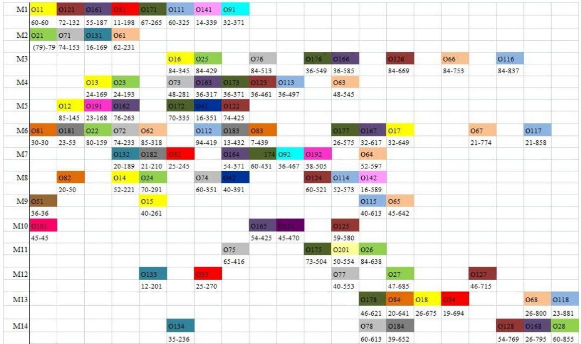
Figure 5.2, decoded solution of the case study in format of a Gantt chart
