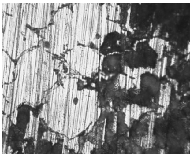
Fig. 3-9 Corrosion morphology of the 20 mm sample was influenced more dominantly by the microstructure as in this micrograph.
