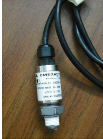
Figure 4.8 Pressure transducer (PTD)
