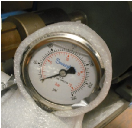
Figure 4.9 Oil-filled pressure gauge
