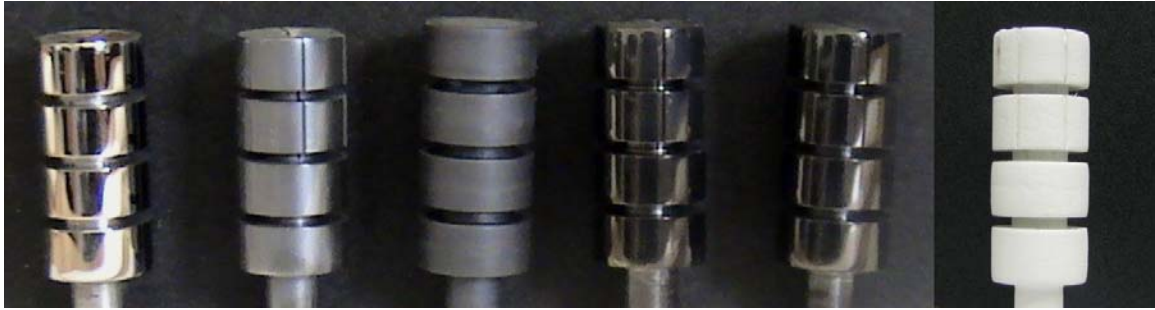
Figure 11 Picture showing the pins used in the order from left to right: the uncoated pin, the S.B. WS2 coated pin, the A.S. WS2 coated pin, the TB 40 coated pin, the TB 41 coated pin, and lastly the BN coated pin
