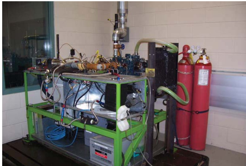
Figure 3.1: Experimental Engine and Fuelling System
