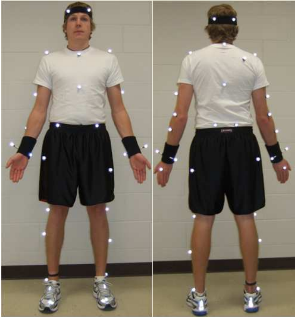
Figure 1- Full body motion capture marker placement of 39 passive reflective markers used for Vicon data collection. Anterior view (left) Posterior view (right).
