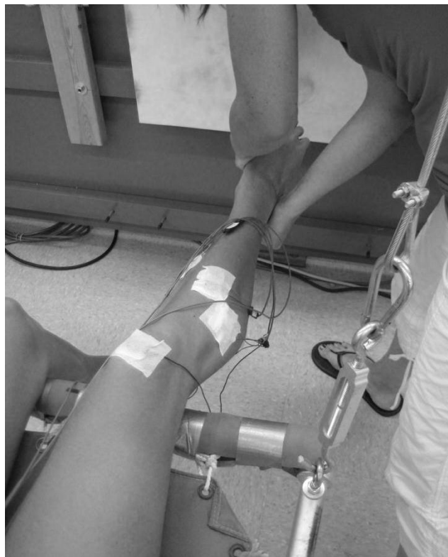
Figure 16: The maximum voluntary exertion (MVE) of the fibularis longus (FL) was taken with the participant lying supine on the human pendulum apparatus. Manual resistance was provided by the investigator to prevent eversion and plantarflexion.
