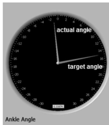
Figure 18. The target ankle angle was displayed on a computer monitor in the participants' field of view during each trial and was monitored throughout the impact. Participants were required to maintain 0%, 20%, 40%, and 60% of their maximum dorsiflexion by aligning the arrows represented on the computer monitor.
