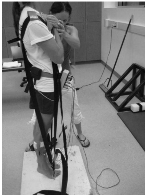
Figure 15: Maximum voluntary exertion (MVE) of the triceps surae group (lateral gastrocnemius (LG), medial gastrocnemius (MG), and soleus (SOL)) was taken by having the participant maximally plantarflex by performing a standing calf raise against padded shoulder straps.
