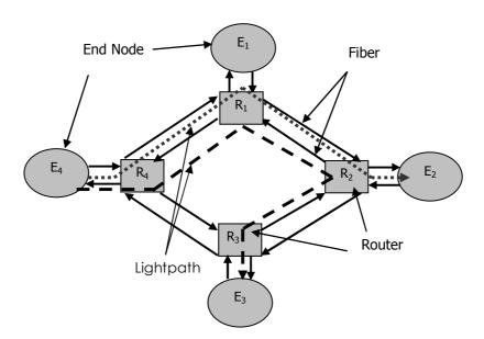
Figure 2.2.8.1: Lightpath shown by dashed-line on Physical Topology
