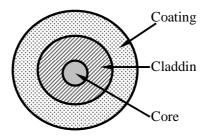
Figure 2.2.1.2: The cross-section of a fiber [21]
