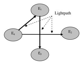
Figure 2.2.8.2: A logical topology drawn from physical topology has shown Fig. 2.2.8.1.
