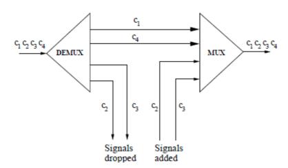
Figure 2.2.4.1: An Optical Add-Drop Multiplexer [21].
