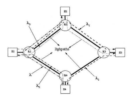
Figure 2.2.2.1: A Wavelength-Routed Network [22]
