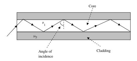
Figure 2.2.1.3: Optical Signal Propagation through a Fiber
