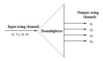
Figure 2.2.3.2: A Typical 4- Output De-Multiplexer [21]
