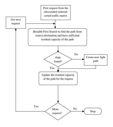
Figure 4.1.1: Generate Initial Logical Topology.
