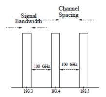
Figure 2.2.2b: Signal bandwidth and channel spacing [21]
