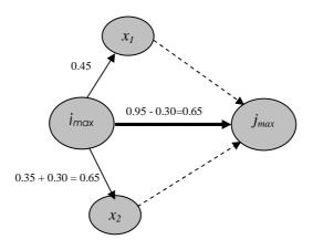
Figure 3.4.3a: Choice 2 - Traffic routing after removing 0.30 units.
