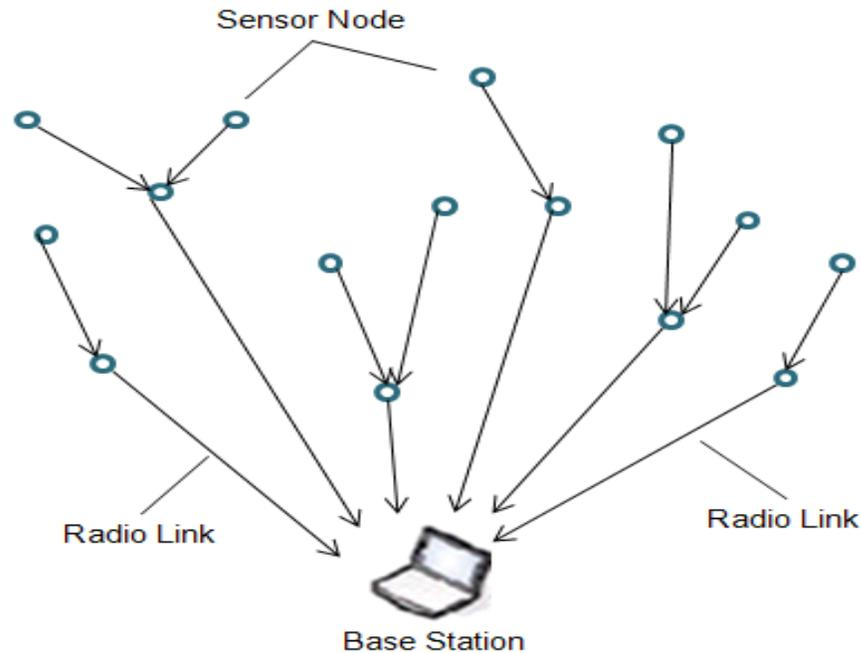
**Figure 2.3** Multi-hop communication of flat architecture
