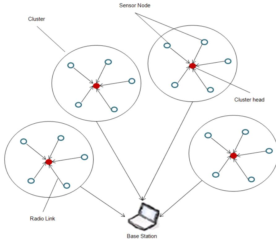
**Figure 2.4** Single-hop communication of hierarchical architecture
