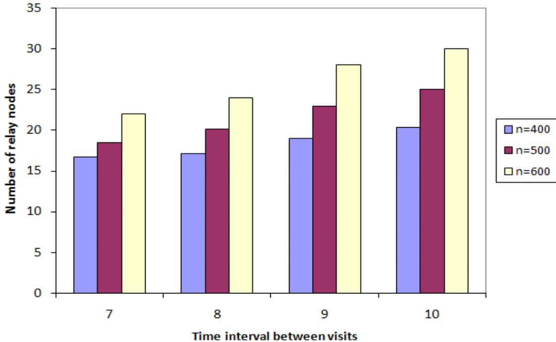
**Figure 4.2** Variation of the number of relay nodes with the variation of  $T_r$ , under various network sizes for the grid setting 165-Grid.
