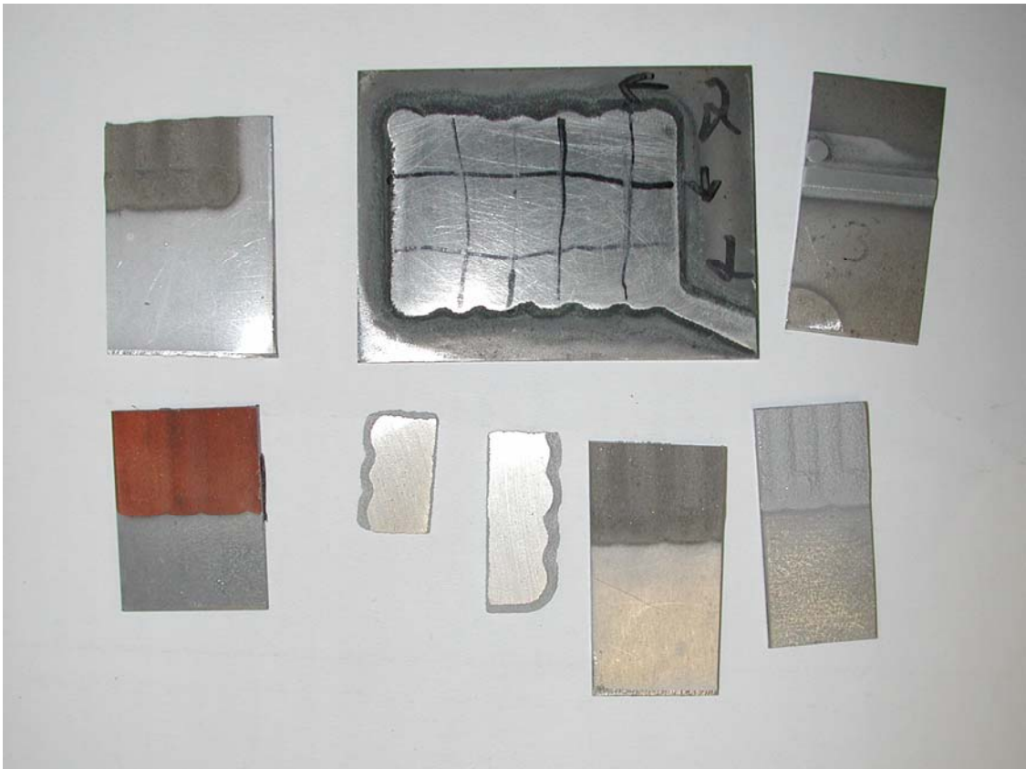
Figure 1.3 Examples of cold sprayed samples for study. (top- left to right nickel composite on aluminum, 2 aluminum composites on steel, bottom- left to right copper composite on steel, 2 pure aluminum, nickel composite on aluminum, aluminum composite on steel)
