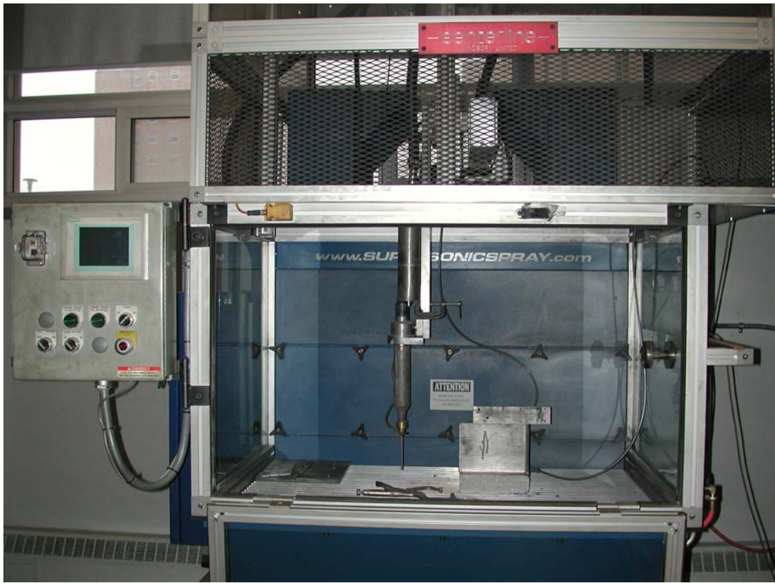
Figure 1.2 Low-pressure gas dynamic spray unit developed by Centerline Limited [2] used to spray all samples.
