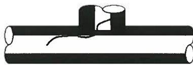
(c) Blowout at Tee
