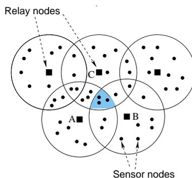
Figure 2.4: Sensor nodes in overlapping coverage area.
