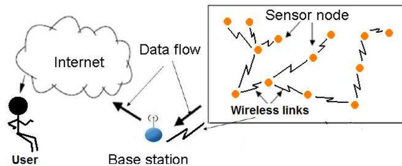
Figure 1.1: A general layout of sensor network
