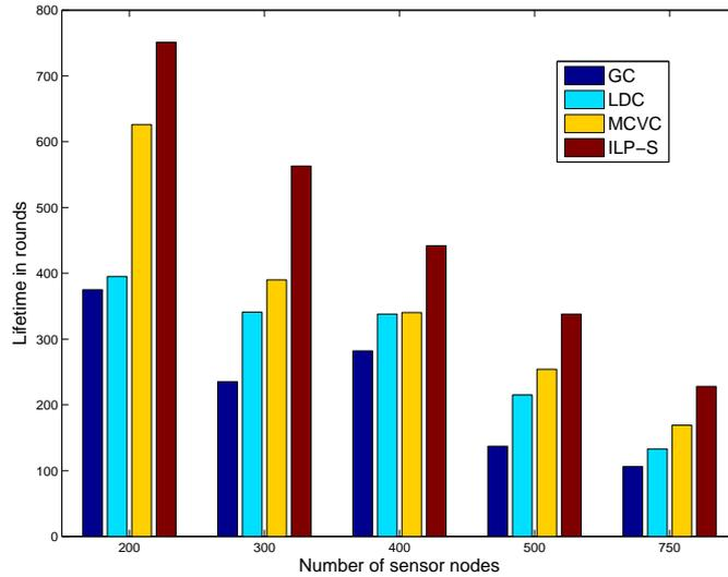
Figure 4.2: Comparison of network lifetimes with different clustering methods for a 24 relay node network under the single-hop routing scheme.
