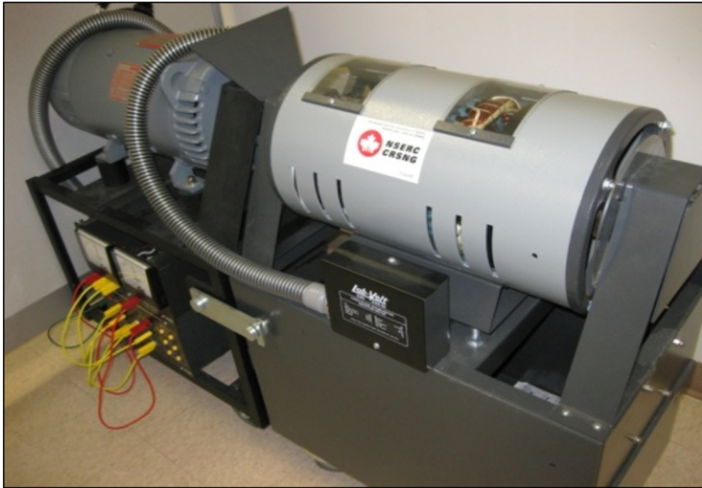
Fig. 3.2. The doubly-fed induction generator (DFIG) under the investigations.
