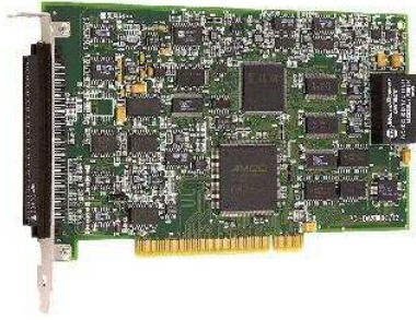
Figure 2.6: PC hosted data acquisition board.
