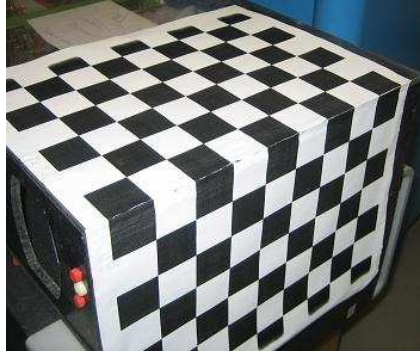
(a) a standard calibration cube for visual cameras
