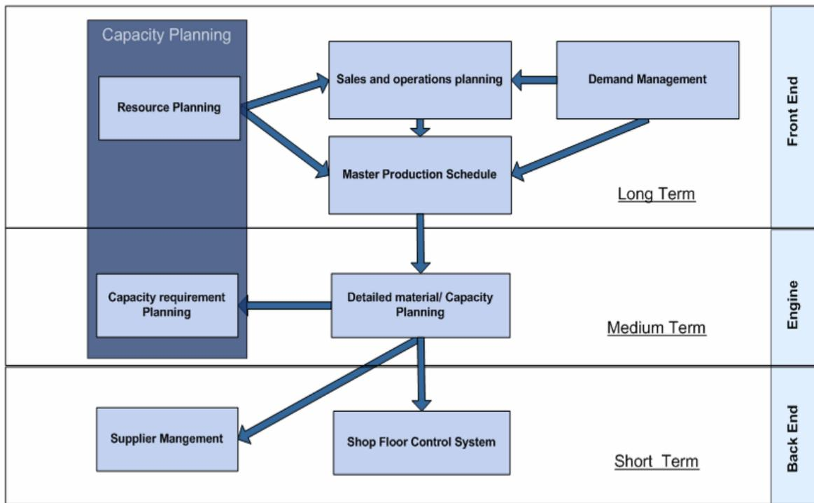
**Figure 1-1: Manufacturing planning and control (Vollman, Berry et al. 2005)**
