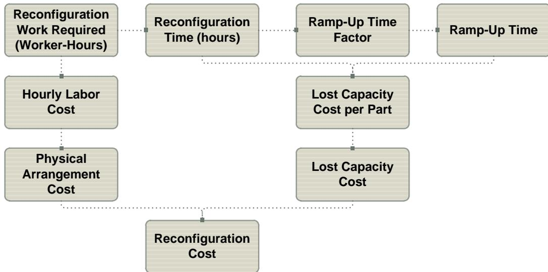
Figure 7-3: Reconfiguration Cost Structure Model Presented by Spicer and Carlo (2007)
