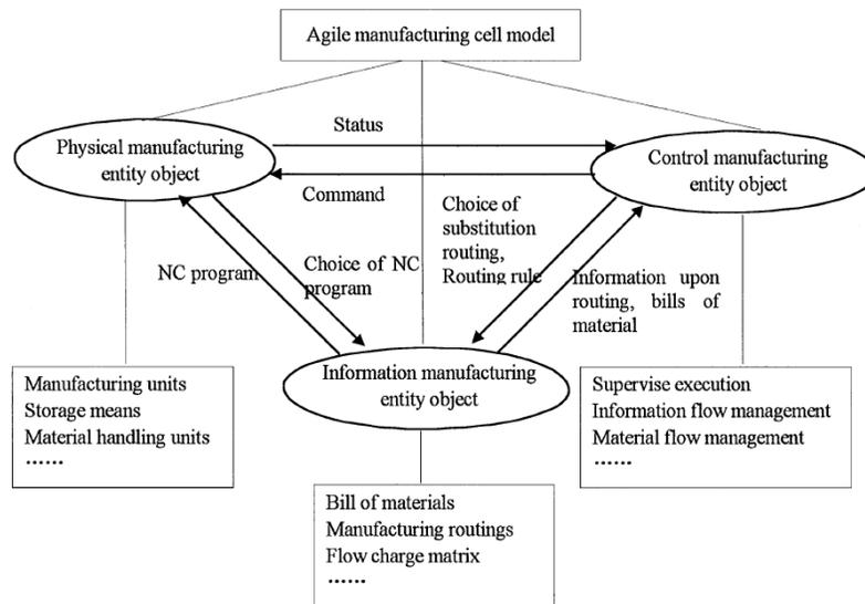
**Figure 2-1: Manufacturing entity objects of an agile manufacturing cell (Zhang and Zhang 1999)**
