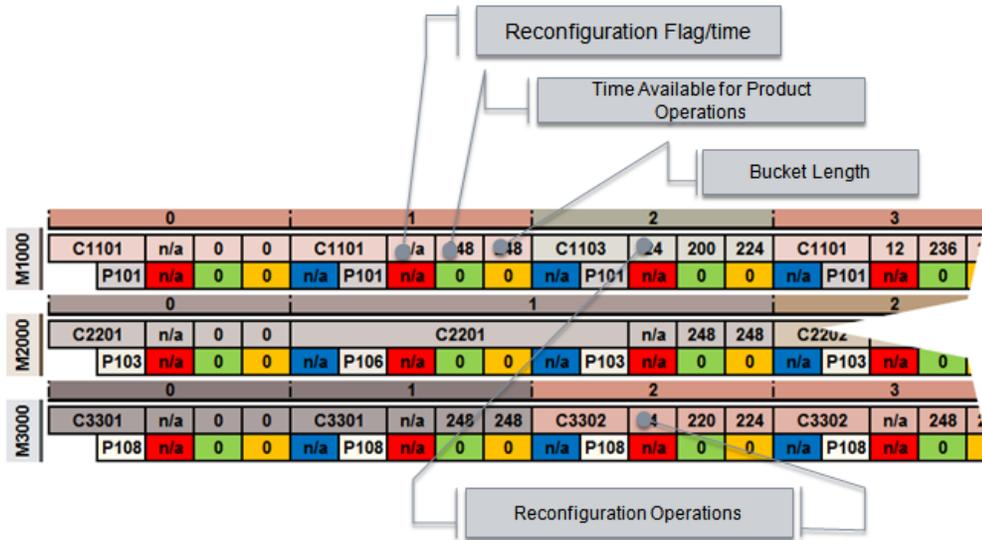
Figure 8-2: Configuration Map Setp#2: Updating Reconfiguration Flags and Times
