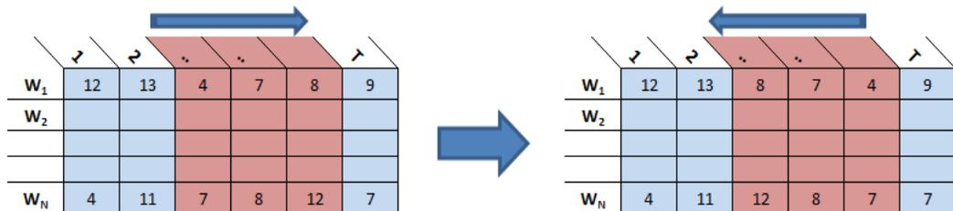
Figure 5-14: Tuple Invert Operator
