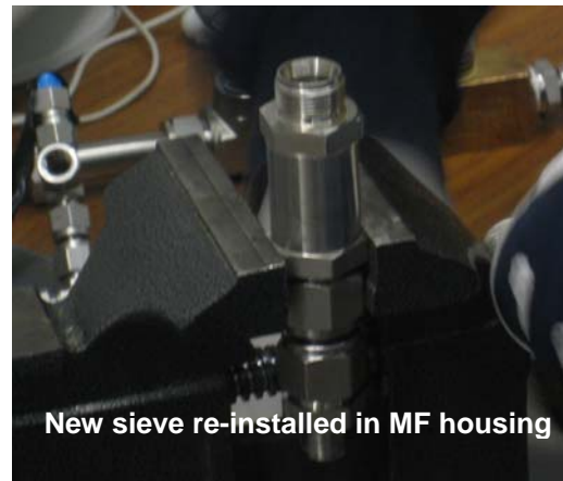
Figure 4.21. Inline micro-filter (MF): (c) Cleaning of filter housing and (d) Filter re-installation.
