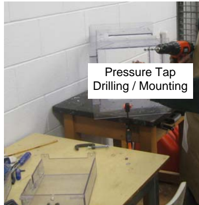
g. Test Chamber Finishing and Assembling-1
