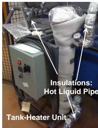
x. Instrumentation and System Insulation-3
