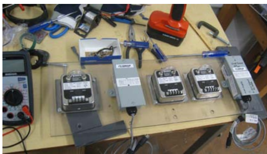
q. Airside Pressure Transducers Panel Making
