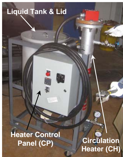
k. Tank-Heater Cart Unit Assembly & Fitting
