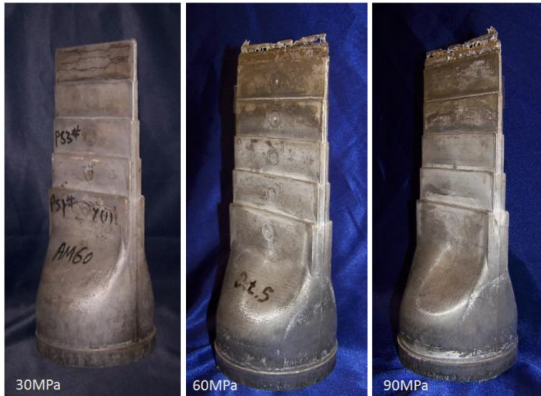
Figure 4- 4. 5-step castings solidifying under applied pressure 30, 60, and 90MPa.
