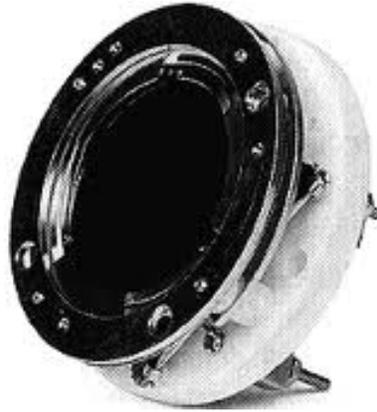
Fig 2 m: A picture of chevron configured 40mm MCP plates manufactured by Quantar Technologies along with the resistive anode encoder. Image courtesy [8].
