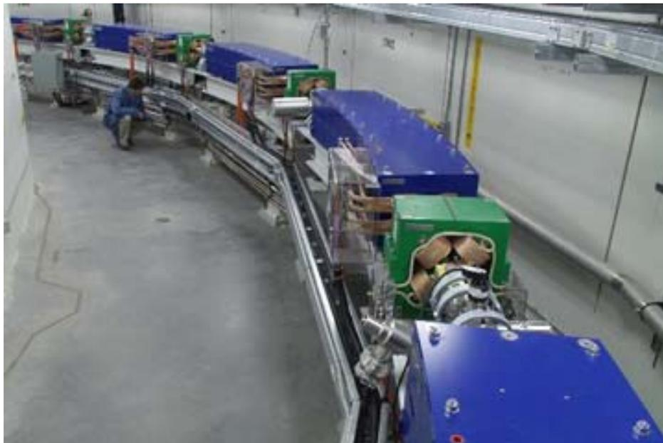
Fig 1 c: Bending magnets are blue colored dipole magnets that are used to guide the electrons around the ring and the green quadrupole magnets are used to force the electron bunches into a fine beam. [Picture Courtesy: Canadian Light Source]
