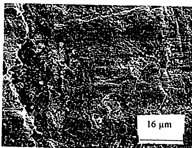
Fig. 4.50 Scanning electron microphotograph (SEM) of PTFE aged in 100 mS/cm saline solution, at 99\pm 2^{\circ}\text{C} , time of immersion 5000 h. (Magnification, 2,000).
