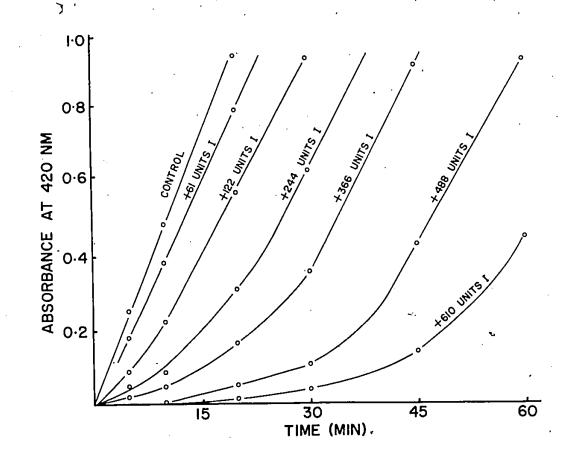
Effect of CaCl<sub>2</sub> and EDTA on inhibitor inactivation.
