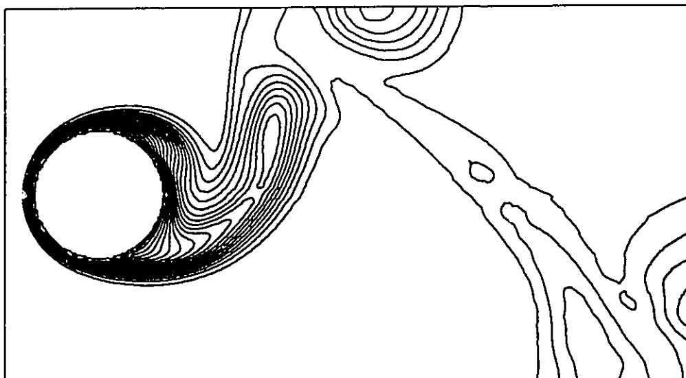
Figure 5.83 Isothermal contours for the case of forced convection (combined oscillation, \tau^* = 0 , a_x = 0.2D , a_y = 0.4D , minimum and maximum contour level: 0.05 and 1, contour interval: 0.05)
