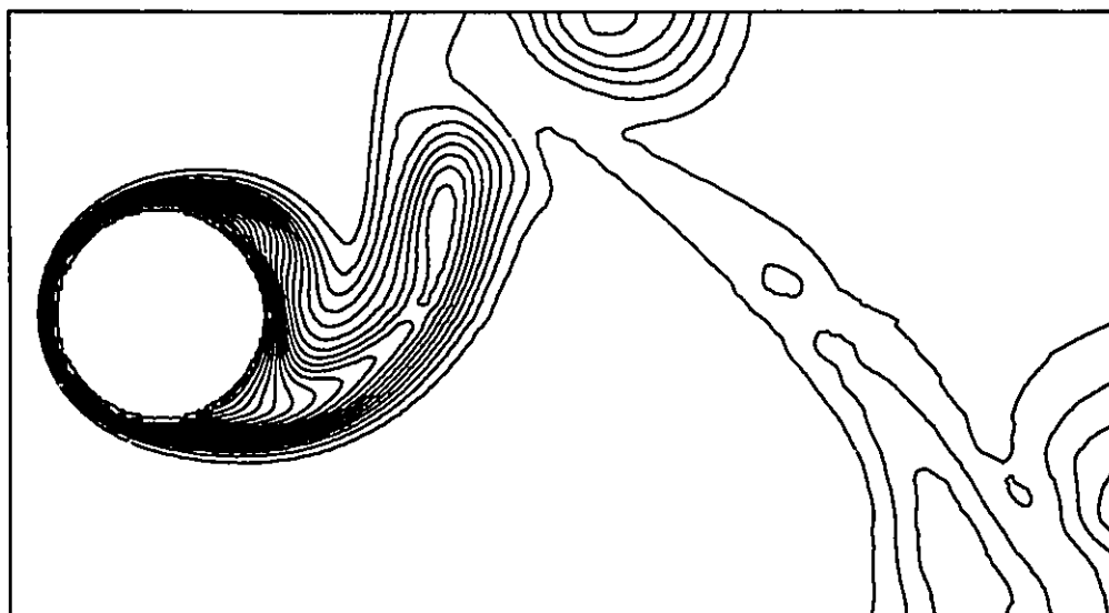
Figure 5.87 Isothermal contours for the case of forced convection (combined oscillation, \tau = 1 , a_x = 0.2D , a_y = 0.4D , minimum and maximum contour level: 0.05 and 1, contour interval: 0.05)
