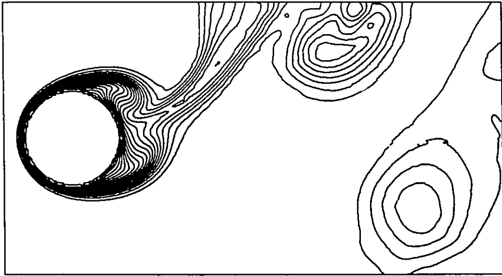
Figure 5.88 Isothermal contours for the case of mixed convection (combined oscillation, \tau^* = 0 , a_x = 0.2D , a_y = 0.4D , minimum and maximum contour level: 0.05 and 1, contour interval: 0.05)
