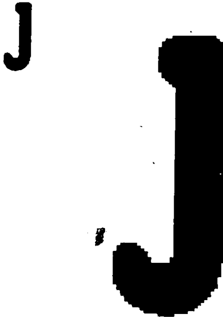
Figure_2.10: Replication method for English character, scalx=4.0 and scaly=4.0, character with one contour.
