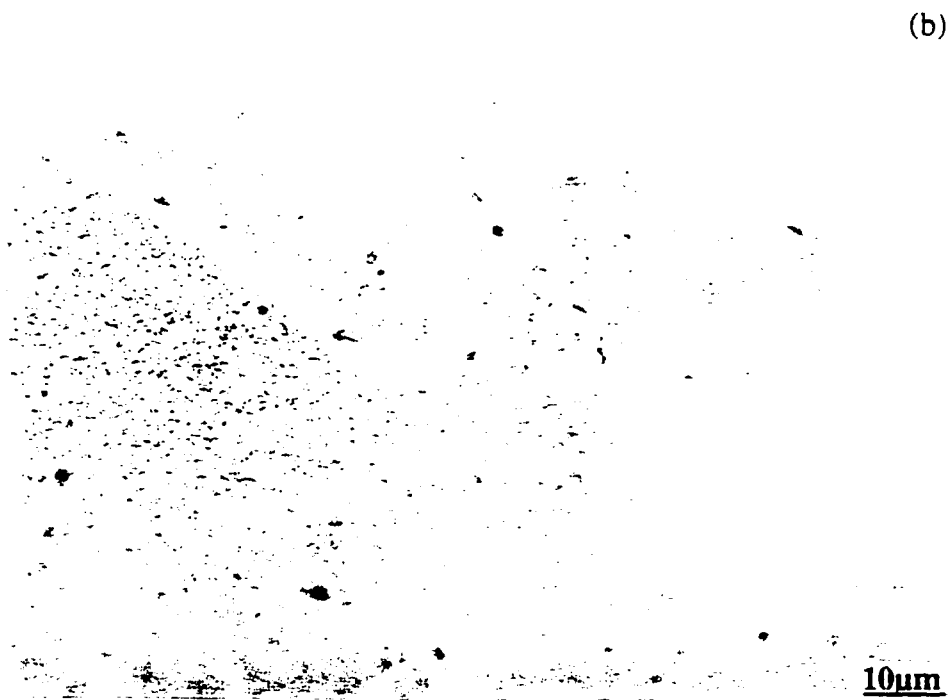
Fig.33 Optical micrographs for the alloys aged at 250°C for 140 hrs: (a) base alloy and (b) 0.4%Be alloy.
