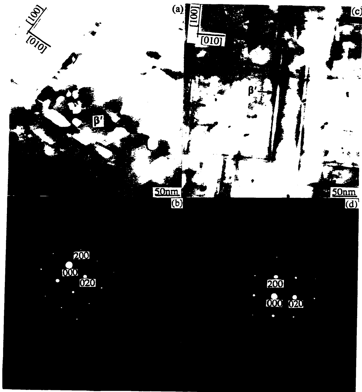
Fig.39 TEM micrograph and corresponding SADP for the alloys aged at 250 °C for 600 min., showing \beta' rods, spots are from the matrix. (a,b) base alloy and (c,d) 0.4%Be alloy. Foil orientation [001] .
