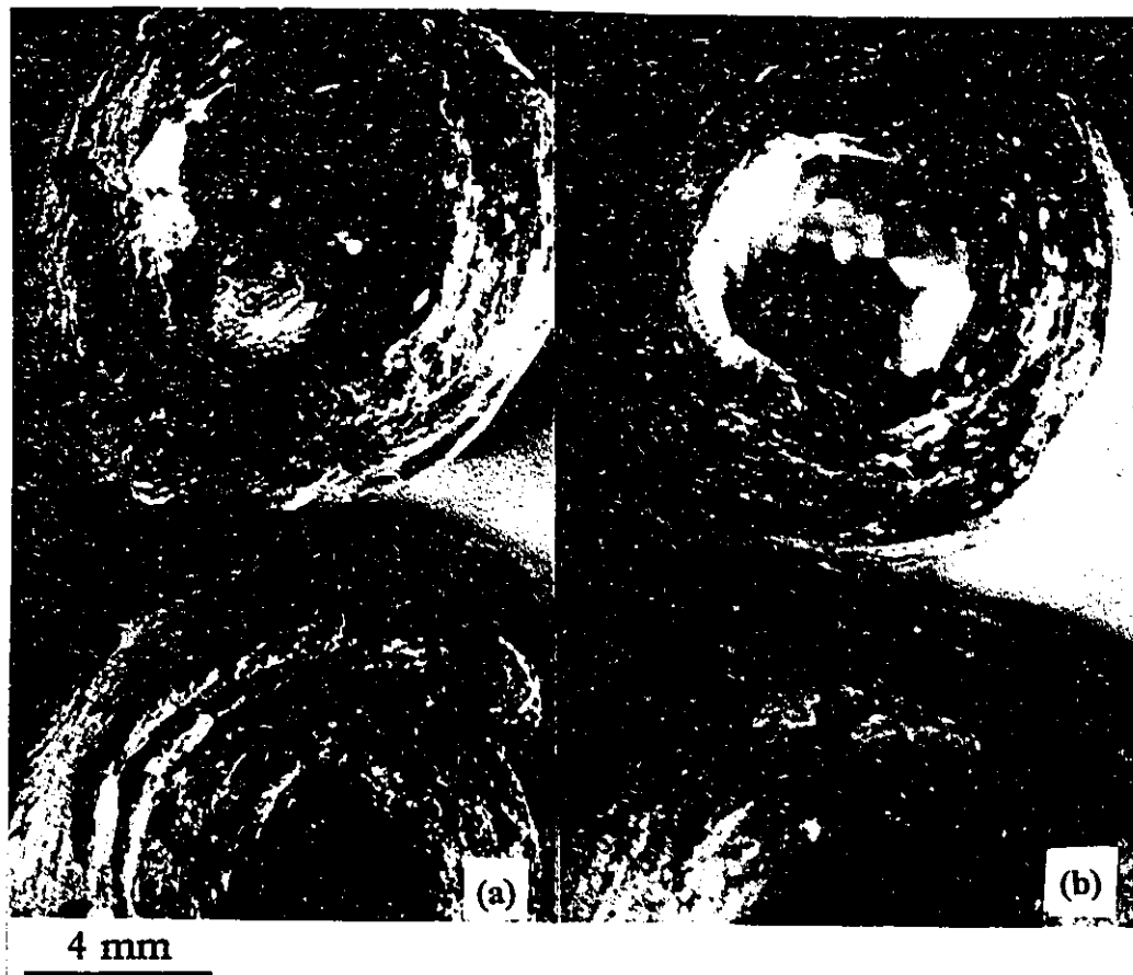
Fig. 4.14. Optical micrographs of worn surfaces of samples (top) and counterfaces (bottom) after sliding at 300°C under 10N load for Al6061 (a) and Al6061-20%Al 2 O 3 (b).
