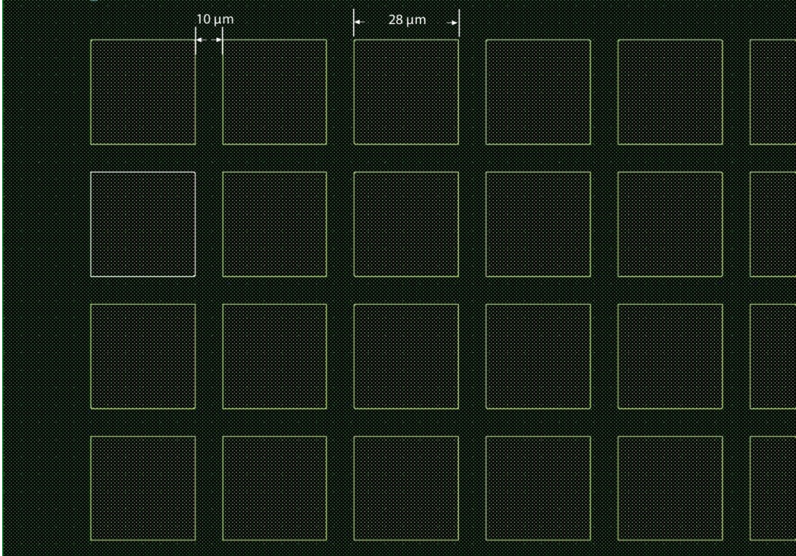
Figure 5-7 Close-up of the mask used to create the cavity
