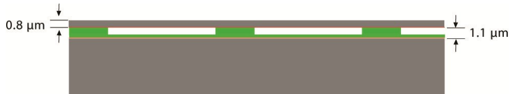
Figure 5-15 CMUT after removal of silicon and BOX layers
