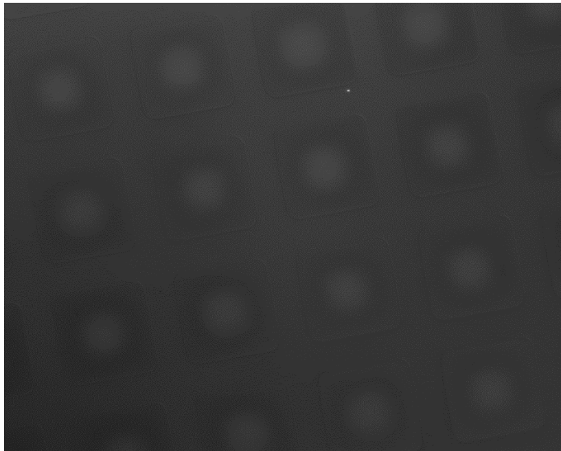
Figure 5-16 SEM image of the CMUTs after silicon removal
