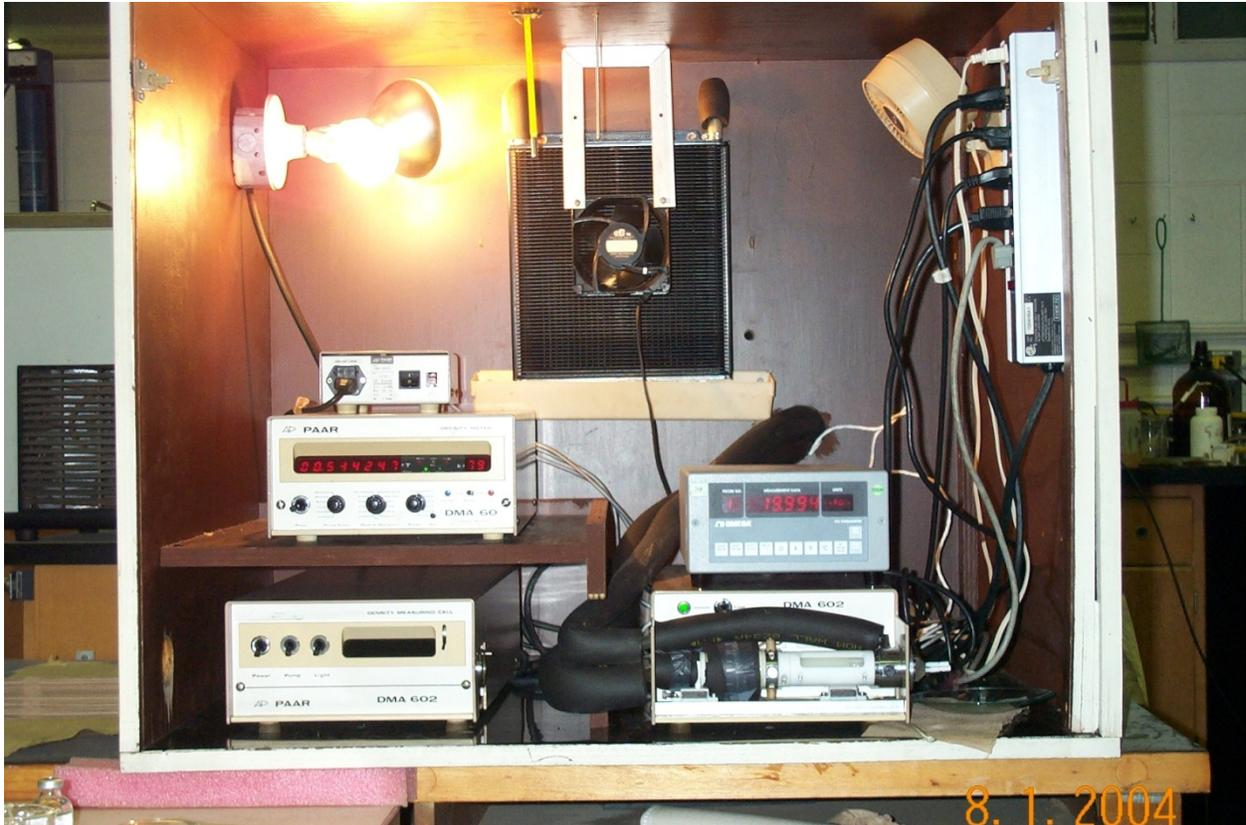
**Figure 3.1:** The Anton-Paar Density Meter Unit and The temperature Control Chamber
