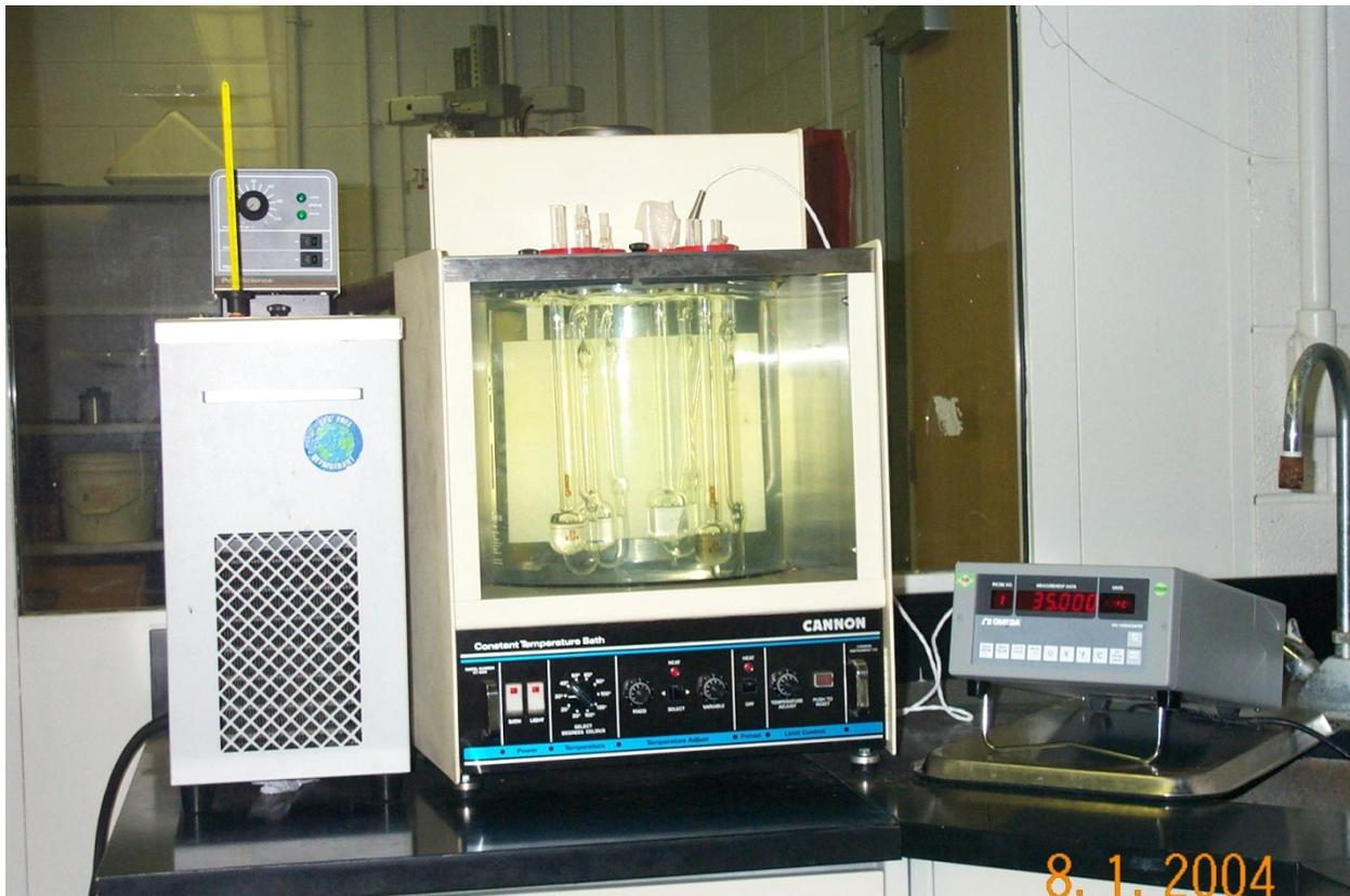
**Figure 3.3:** The CT-1000 Viscosity Bath and the Omega Precision Thermometer
