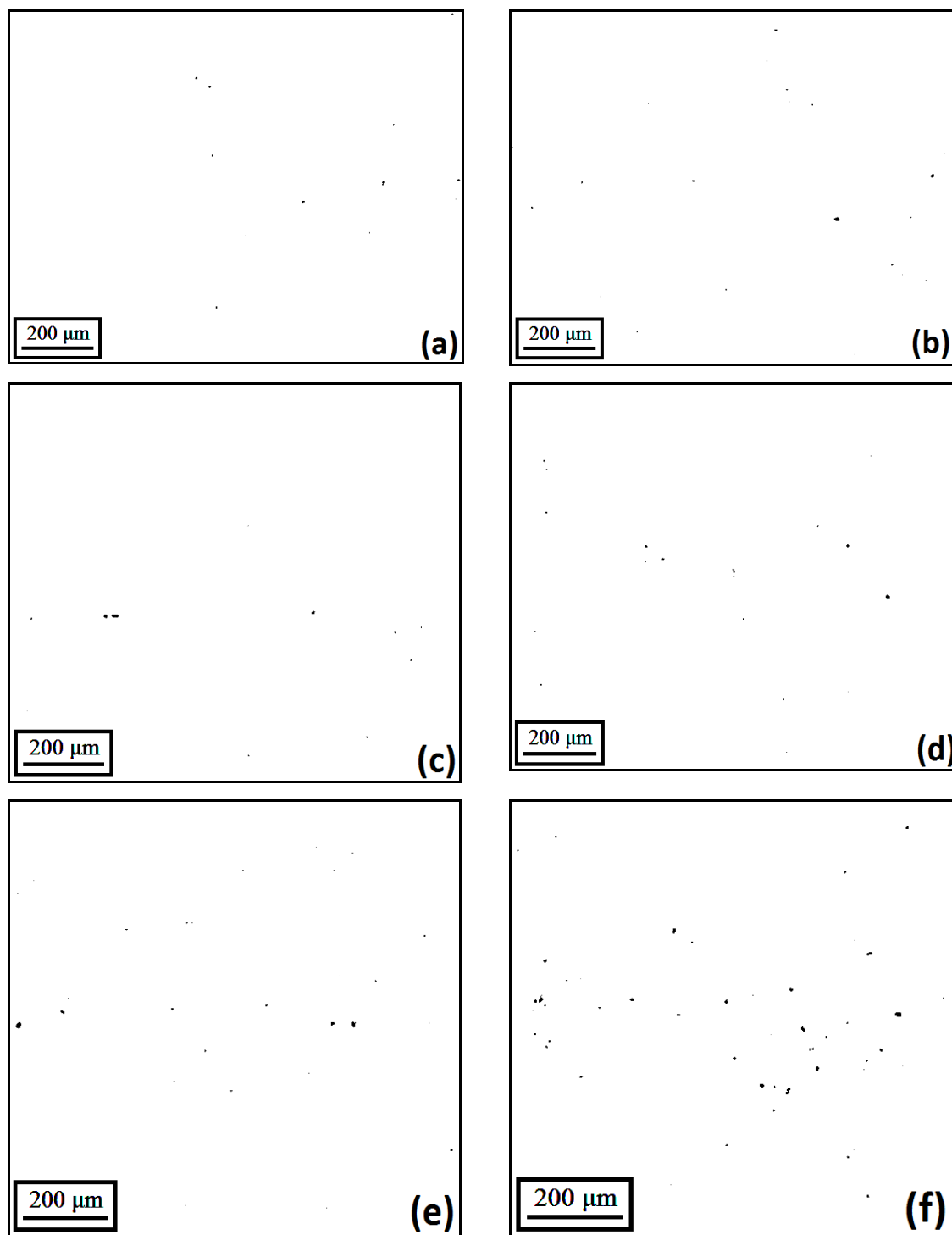
Figure 7-5 Voids in DP500 EHF specimen at strain: (a) 0.1, (b) 0.2, (c) 0.3, (d) 0.4, (e) 0.5, and (f) 0.6 (mm/mm). Black spots are the voids in the white matrix.
