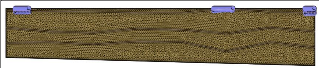
Figure 3.3a: Boundary condition for mass-transport showing the location of the contaminant source in the south-north model
