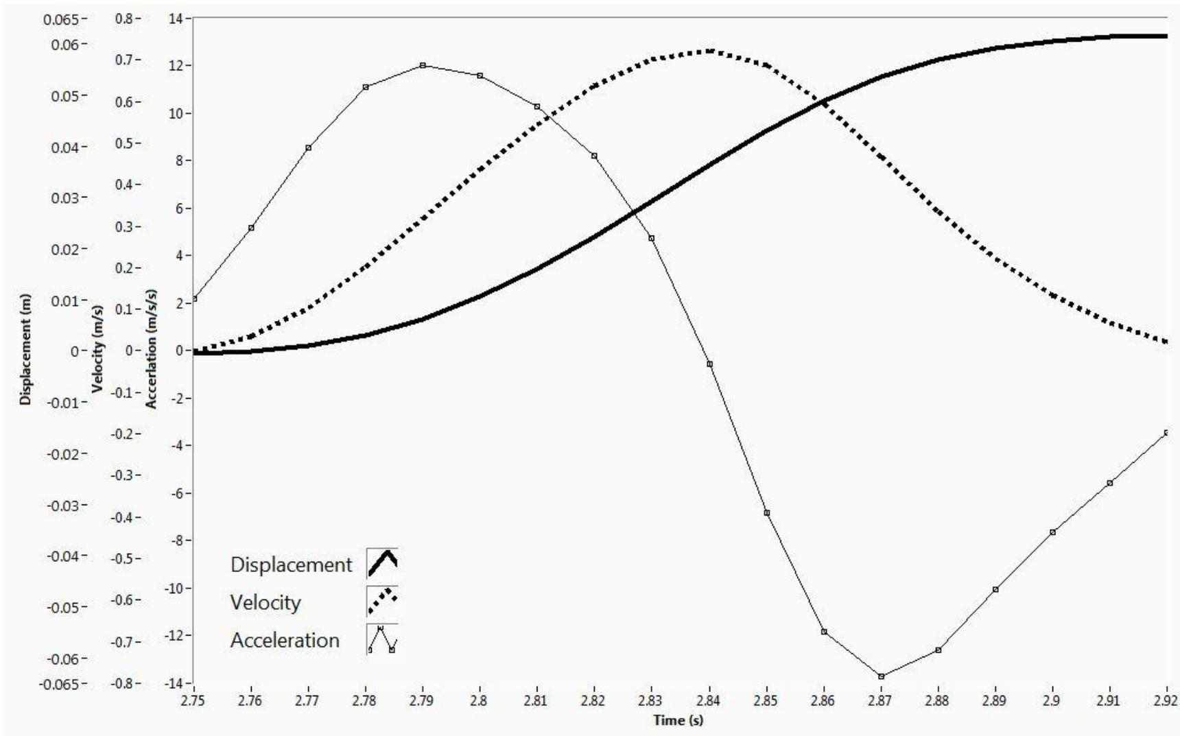
Figure 11. An example of the perturbation motion caused by the robotic platform during a perturbation in the back direction for VG. The robot is programmed to move a total of 0.065 m in a 0.17 second period. The resulting velocity and acceleration profiles are shown for the given robotic platform motion.
