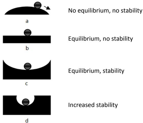
Figure 3. Degrees of stability (Reeves & Cholewicki, 2003). Diagram *a* is a system that has no equilibrium and no stability. Diagram *b* is a system that has equilibrium but no stability. Diagram *c* is a system that has equilibrium and is stable. Diagram *d* is a system that has increased stability in comparison to the previous diagrams.
