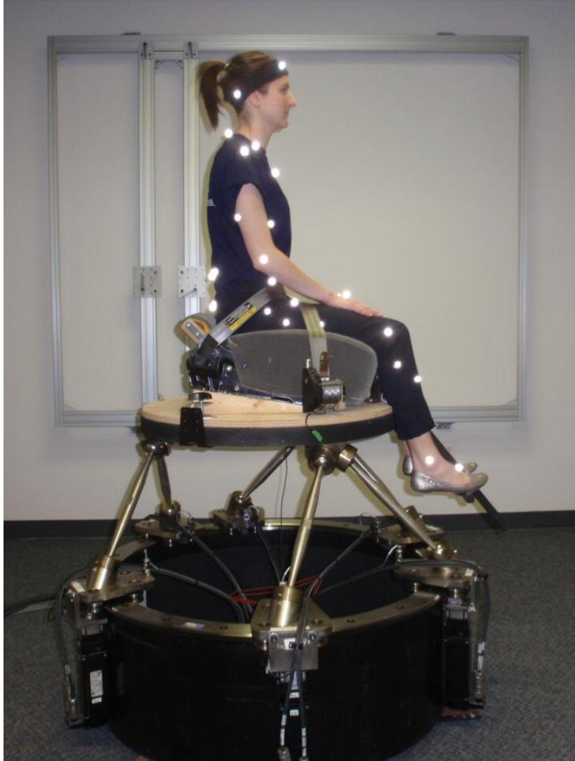
Figure 14. Participants were seated on a backless car seat and told to maintain neutral posture during both the pre-perturbation and perturbation protocols.
