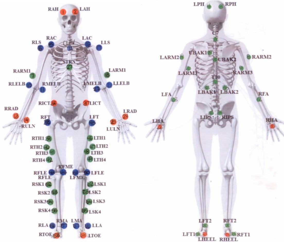
Figure 8. Marker set as it was applied to participants for the passive motion capture. There were 72 markers altogether.
