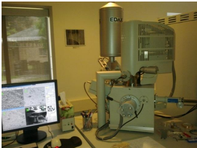
Figure 3.5 Scanning electron microscopy used in research objective from Great Lakes Institute for Environmental Research at University of Windsor
