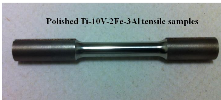
Figure 3.11 Schematic presentation and real image shown of a tensile test sample
