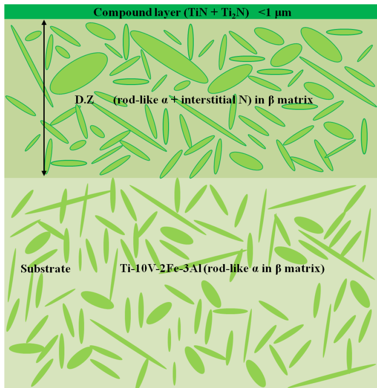
Figure 5.2 Schematic presentations of the ion nitrided Ti-10V-2Fe-3Al microstructure consisting of a thin compound layer and thick diffusion zone.
