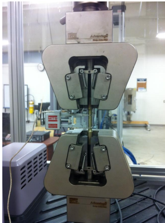
Figure 3.13 Uni-axial tensile testing on Ti-10V-2Fe-3Al using MTS Criterion Model 43 tensile testing machine with loading rate of 0.5 mm/min.
