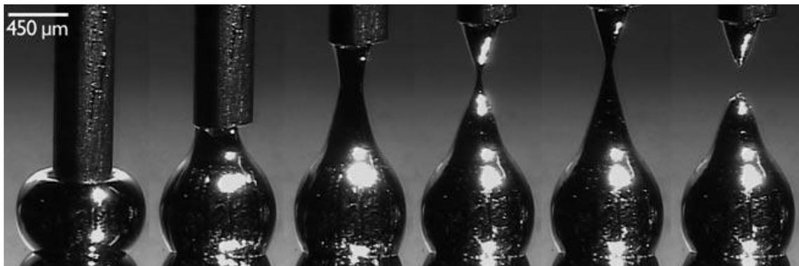
**Figure 1.17.** A series of photographs of the formation of a conical tip of EGaIn. Adapted with permission from reference 180.
