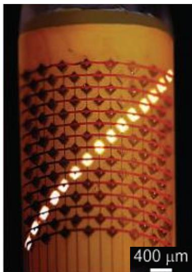
**Figure 1.07.** Photograph of the operating display after the alignment of the top electrode. The display contains 113 LEDs that are assembled in an interleaved fully addressable array. Adapted with permission from reference 79.
