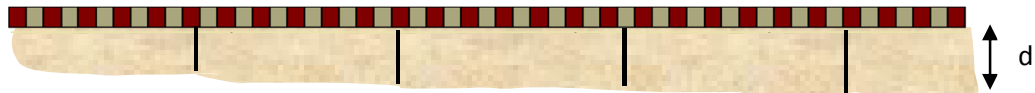
Fig.3. 2. Schematic scattering layer with random phase shifting technique. Each section has random phase shift ( 0-2\pi ) and the number of section could vary due to shape of the lower boundary
