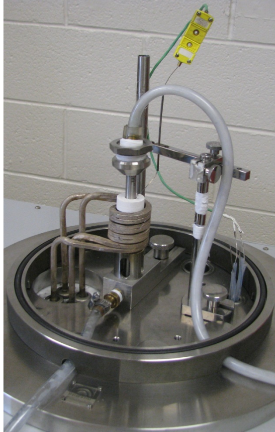
Figure 14 - UMSA configuration for rapid liquid quenching.
