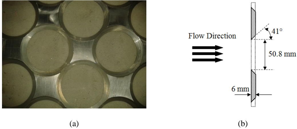
Figure 2: (a) Orificed perforated plate photo (looking upstream), (b) Cross-section of the OPP
