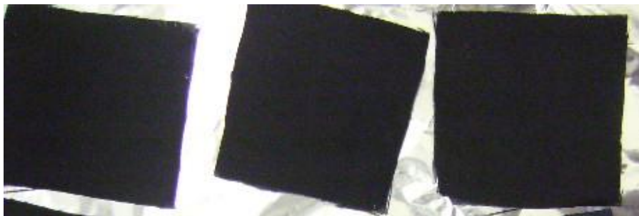
Figure D2 Digital picture showing carbon cloth pasted with a carbon base layer.
