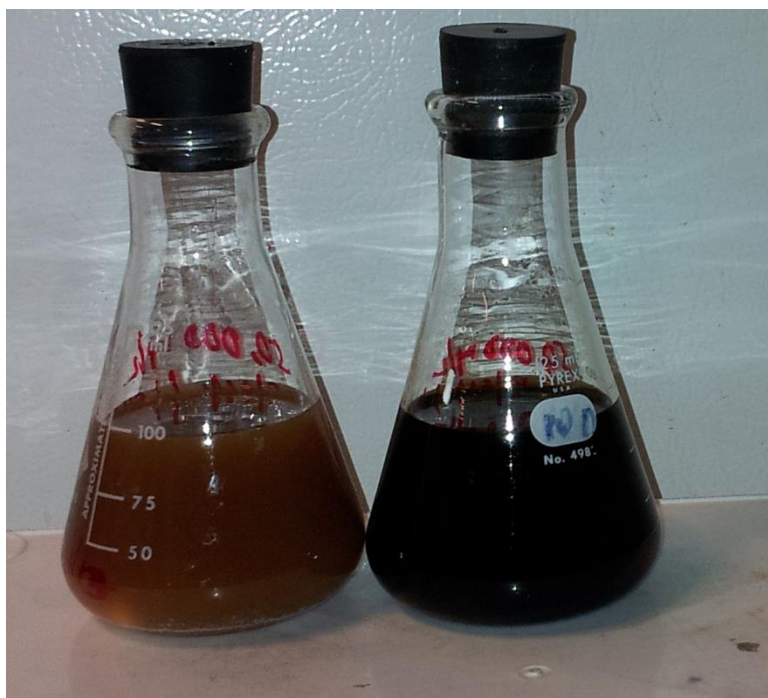
Figure C1 Digital picture showing the color of 50,000 mg L -1 black liquor (5 g black liquor diluted to 100 mL using DI water) a) without pH adjustment (right) b) pH adjusted to 7 (left).
