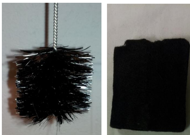
Figure 4.4 Digital picture showing: a) Graphite fiber brush anode and b) Graphite felt anode used in SCMFCs.
