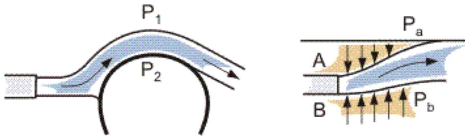
**Figure 2.3: Coandă effect; on the left streamline curvature, on the right restricted entrainment [10]**
