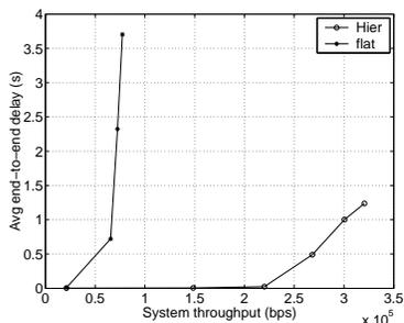
Fig. 3. Delay vs. throughput for 40 communication pairs
