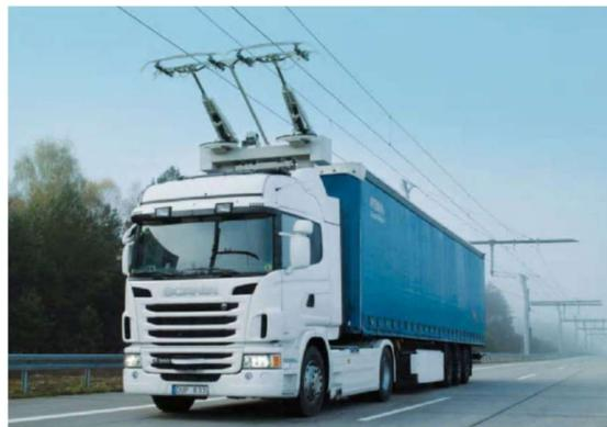
Figure 5. Heavy goods vehicle using electrified highway near Sandviken, Sweden (Alaküla and Márquez-Fernández, 2017.)
