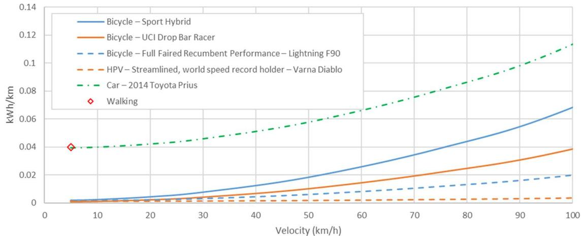
Figure 3. Energy per distance of four different bicycles as a function of speed.
