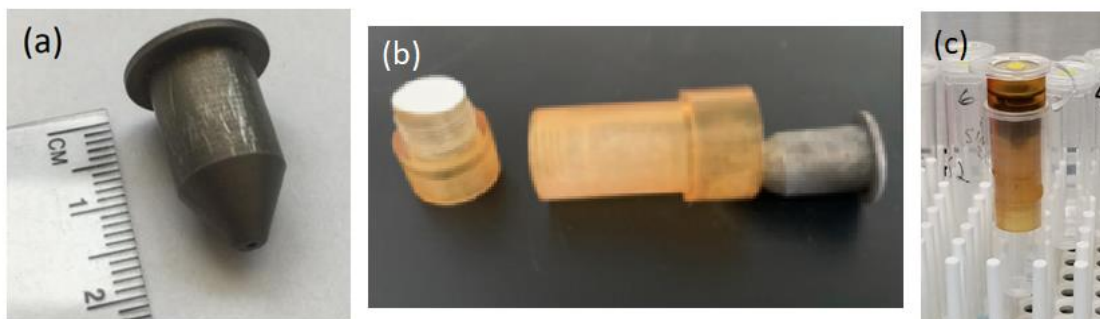
Figure 3.10: (a) Metal cone for rapid concentration of bacteria, shown next to ruler to give approximate size. (b) Centrifuge insert shown before assembly. A filter is placed on the bottom piece of the centrifuge insert before it is assembled. (c) The assembled centrifuge insert with cone is placed in a centrifuge tube.
