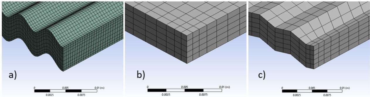
Figure 5. Specified mesh used in the simulation of the (a) sinusoidal (b) rectangular, and (c) triangular beds.
