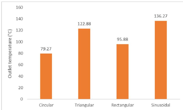
Figure 6. Average outlet temperature for different channel shapes.
