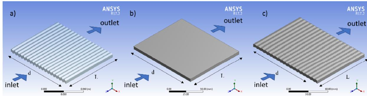
Figure 4. Geometry used in the simulation (a) Sinusoidal (b) Rectangular (c) Triangular.
