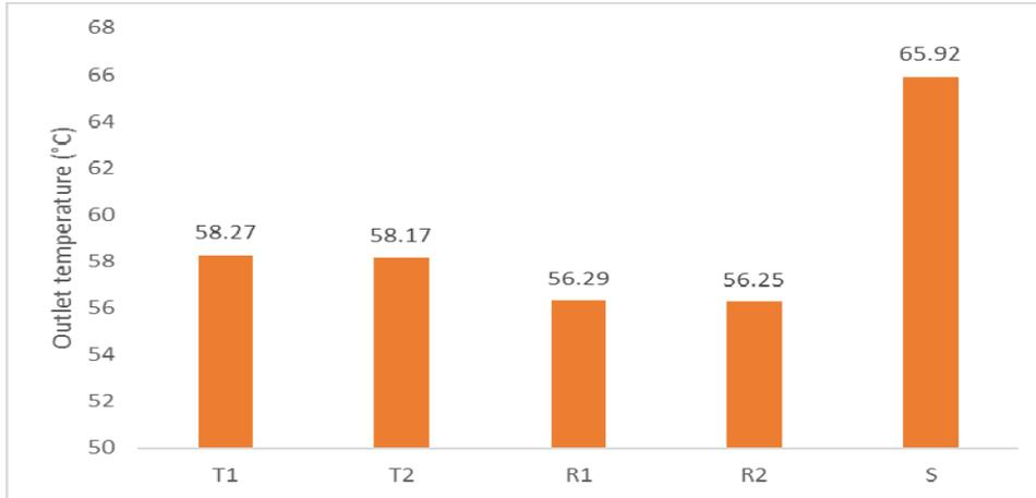
Figure 7. Average outlet temperature for triangular 1 (T1, same dimensions as the sinusoidal), triangular 2 (T2, same surface area as the sinusoidal), rectangular 1 (R1, same dimensions as the sinusoidal) and rectangular 2 (R2, same surface area as the sinusoidal).
