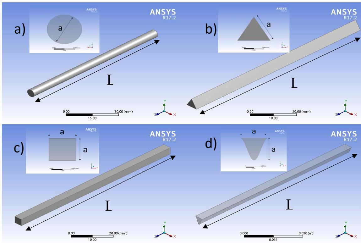
Figure 1. Geometry used in the simulation (a) Circular (b) Triangular (c) Rectangular (d) Sinusoidal.
