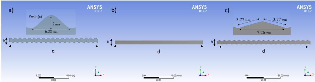
Figure 3. Cross-section schematic of modelled beds. (a) Sinusoidal (b) Rectangular (c) Triangular.
