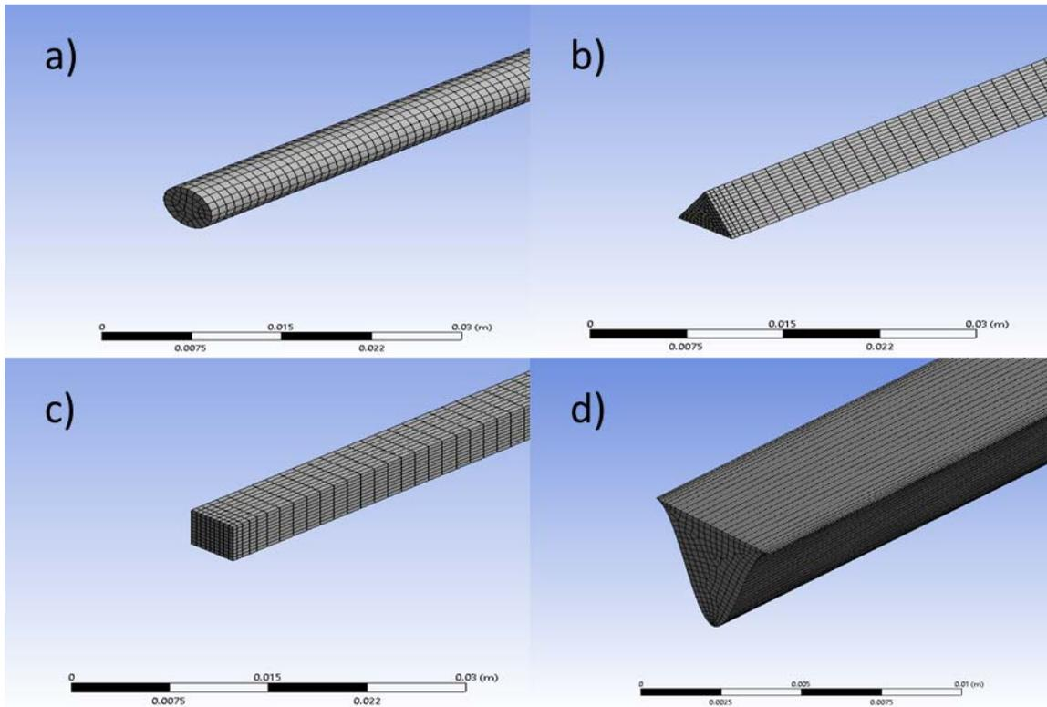
Figure 2. Specified mesh used in the simulation (a) Circular (b) Triangular (c) Rectangular (d) Sinusoidal.
