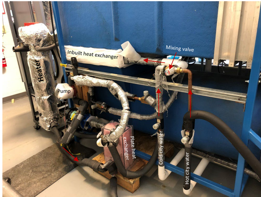
Figure 3.3. Inbuilt heat exchanger air temperature control loop
