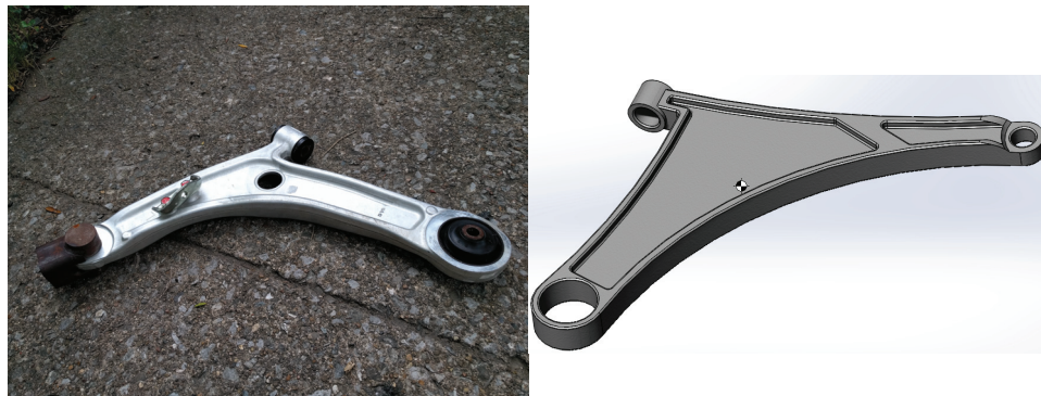
Figure 2.2: Actual lower control arm and CAD drawing
