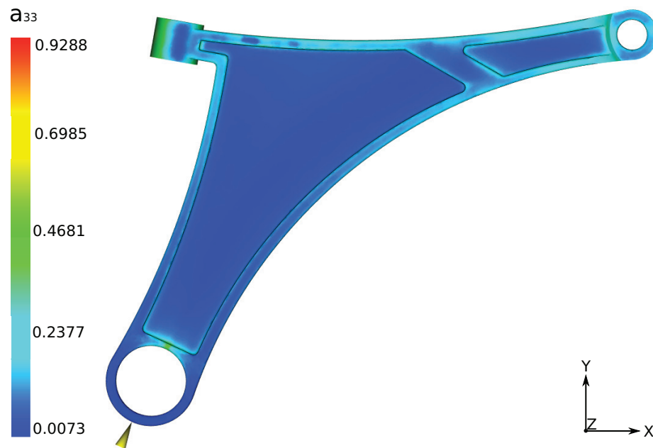
Figure 3.19: Fibre Orientation Result a_{33} with Injection Point Location at Rear Bushing Side. Note that the small a_{33} value throughout the part indicates a nearly planar fibres orientation.
